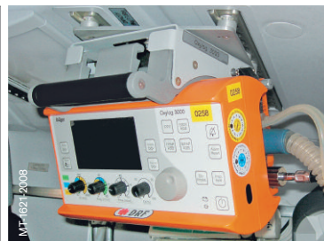
Figure 3: Custom made mounting solution for Oxylog® 3000
