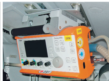
Figure 3: Custom made mounting solution for Oxylog® 3000
